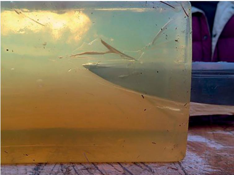
FIGURE 17 Results of a stab into ballistics gel (Author's photo).
