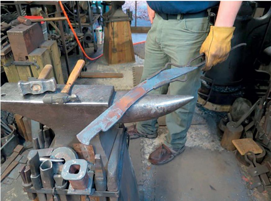
FIGURE 12 The replica *kopis*, after three cycles of heating in the forge and hammering (Author's photo).
